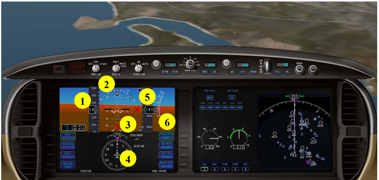
Figure 37 – Cirrus instrument panel. (1) Airspeed indicator: Knots (2) Bank angle indicator: degrees (3) Pitch ladder: degrees (4) Magnetic Headings indicator (5) Altimeter: feet (6) Vertical Airspeed indicator: feet
