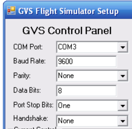
Figure 25 - GVS device default RS-232 connection settings.
